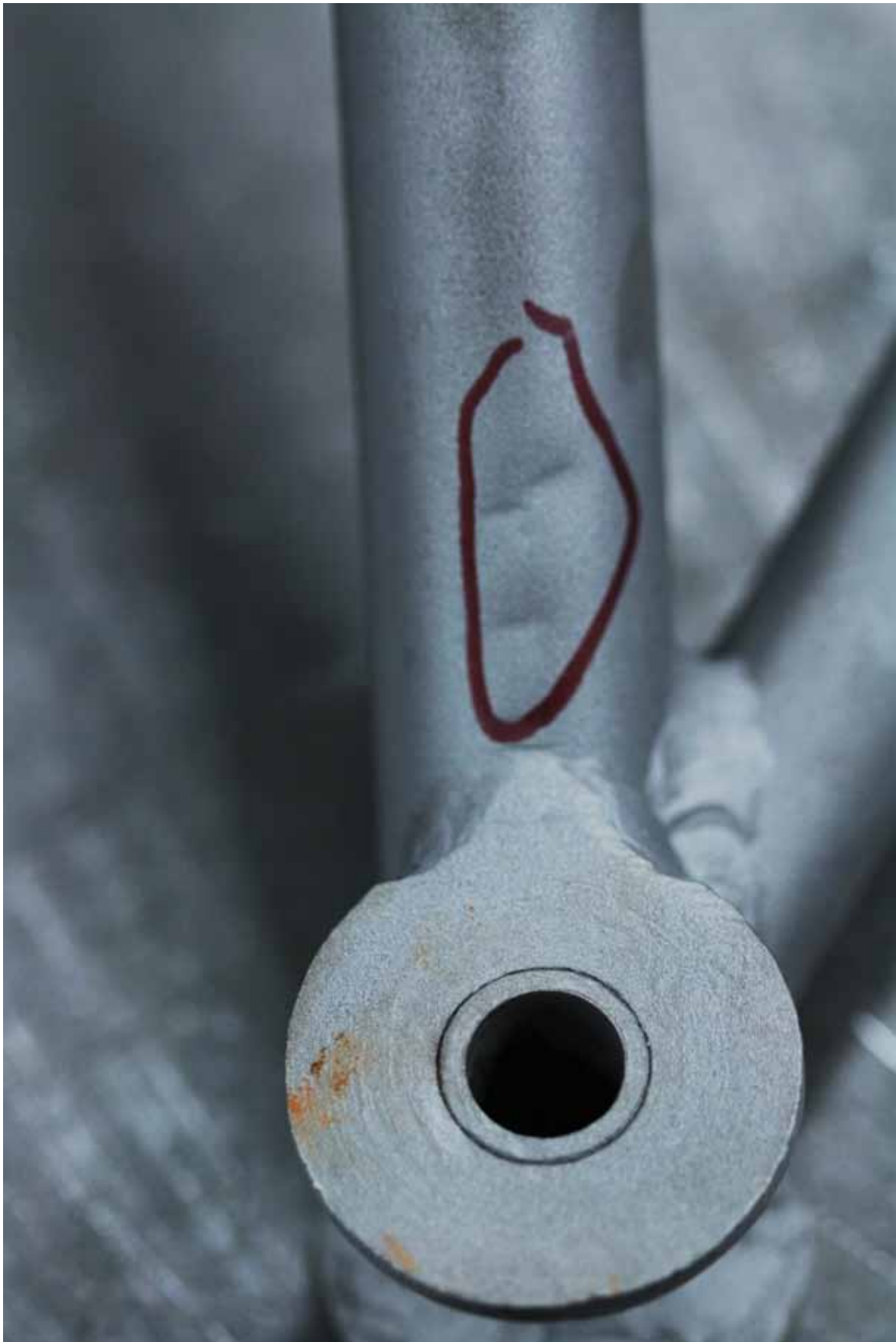
Dents are repaired during the Loree Air rework. According to Steve Loree, the circular slot around the bolt hole is how moisture—a cornerstone of the rust process—enters the tubing in the mount. Loree seals this slot during rework.
